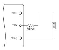
Figure 16. Circuit to Decrease Output Voltage
