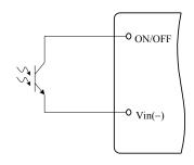
Figure 13. Opto Coupler Enable Circuit
