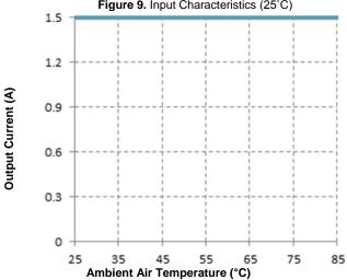
Figure 11. Current Derating Curve under Nature Convection (Ref. Fig. 12 for Airflow Direction; typical Vin, open frame unit, soldered interface)
