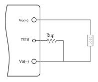
Figure 17. Circuit to Increase Output Voltage
