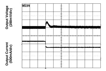
Time - t (200µs/div) Figure 7. Transient Load Response (typical Vin, load current steps from 50% to 25% at a slew rate
