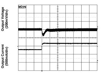
Time - t (200µs/div) Figure 8. Transient Load Résponse (typical Vin, load current steps from 50% to 75% at a slew rate  $0.1A/\mu s$ )
