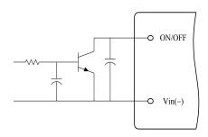
Figure 14. Open Collector Enable Circuit
